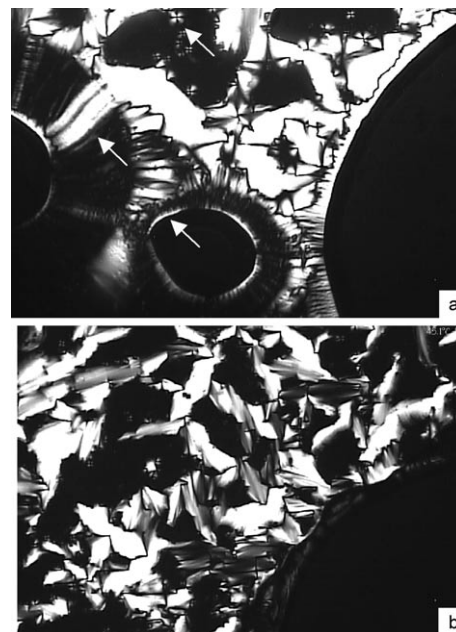
Figure 1. Defect textures of the smectic A phase of 6,6'-di-O-octanoylsucrose, 2a , (x100); a) the oily streak texture and fanlike defects around air bubbles, b) the focal-conic defect and homeotropic textures.
